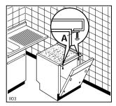
Secure the dishwasher to the counter on the front part by means of two 4,2x13 screws provided (see fig. - point A).
